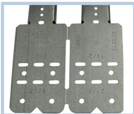
Markings on the bracket ensure the boxes and fittings are set to the correct depth and position between the studs allowing for fast, very accurate and neat installation. Multiple boxes up to a depth of 54mm can be mounted on each bracket. Frequently spaced pilot holes allow boxes and fittings to be easily attached with self tapping screws using only a screwdriver.
